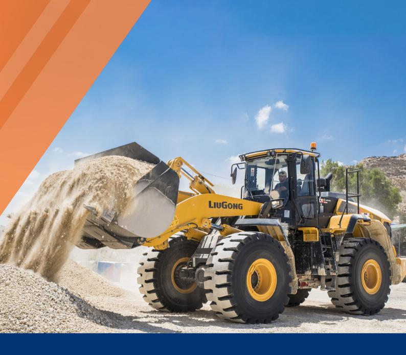
EngineCummins6LTAA8.9Rated Power205 kW (275 hp / 279 ps) @2,000 rpmOperating Weight23,974 kgStandard Bucket Size4.2 m³Standard Breakout Force203 kNStandard Dump Clearance3,151 mm
