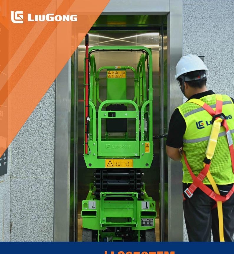
Working Height Max. Overall Lift Capacity Max. Overall Width Overall Length Overall Weight 6.5 m (21'4") 240 kg (529 lb) 0.76 m (2'6") 1.49 m (4'10") 895 kg (1,973 lb)
